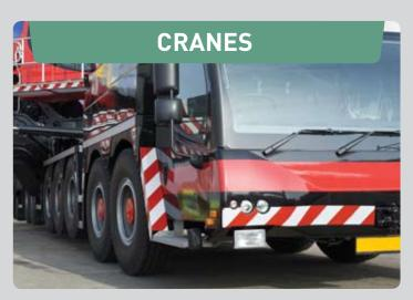
Crane engines are housed in compartments not easily viewed by the driver. LVT's fire suppression system protects the engine against fire caused by escaping fuel or hydraulic liquids.
