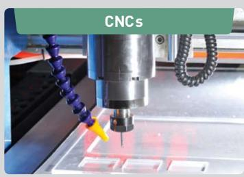
CNC machines processing stainless steels or light metals run the risk of the materials or cooling oil igniting as a result of blade breakage during operation. The linear heat detector withstands chemicals used in the machine's cooling system. The pneumatic systems don't require an external power source.
